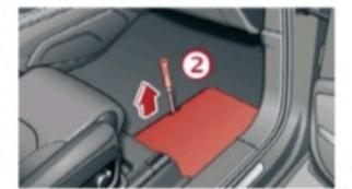
② Lift off the battery compartment cover.
