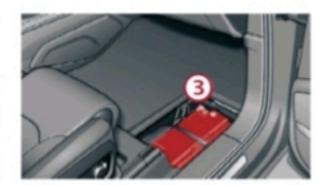
③ First disconnect the negative terminal (-) and then the positive terminal (+) of the vehicle electrical system battery.
