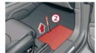
② Lift off the battery compartment cover.
