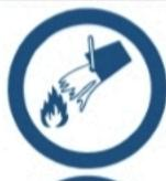
Use large sustained volume of water for lithium-ion battery related fire.
