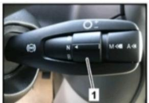
Turn the transmission selector switch (1) to position N.
