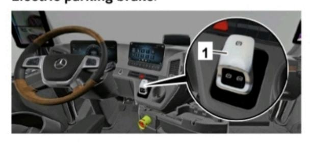
Pull parking brake lever (1) upward. The electric parking brake is engaged.
