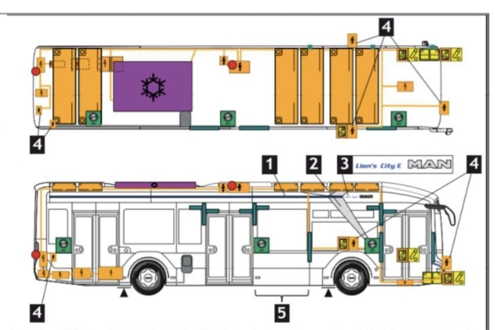
The vehicle type 12C (length 12.185 m) is shown above. For vehicle type 10C (length 10.575 m), the marked skeleton segment  $\frac{1}{2}$  in front of the middle step unit is omitted. Vehicle type 10C may be equipped with two or three battery modules in the front roof
