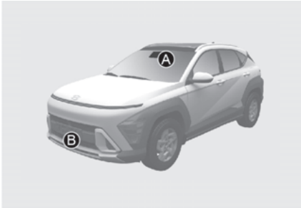
[A] Front view camera [B] Front radar
