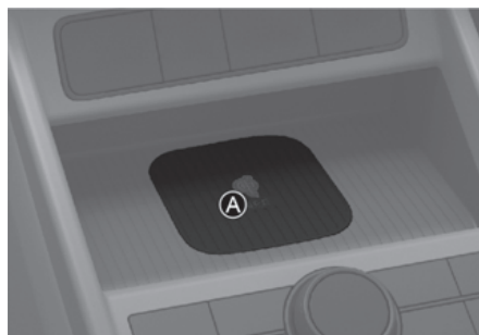
[A] Vehicle authentication pad (Wireless charging pad)
