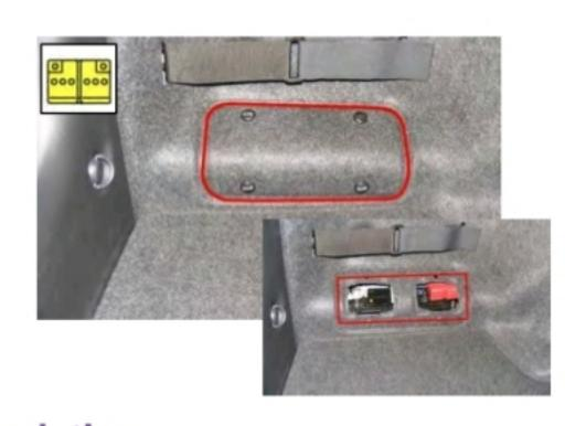
If the 12 Volt battery can not be disconnected, the supplemental restraint systems continue to be active!
