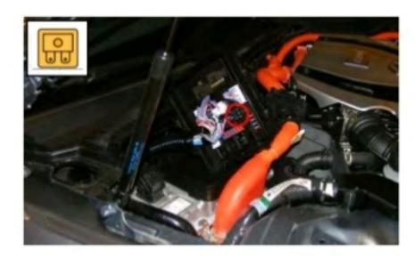
Disconnect the 12 Volt battery. Ground cable first.
