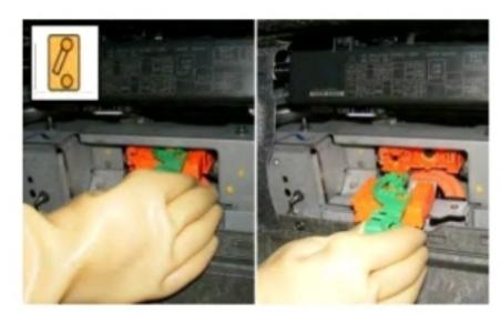
3. Disconnect the 12 Volt battery. Ground cable first.
